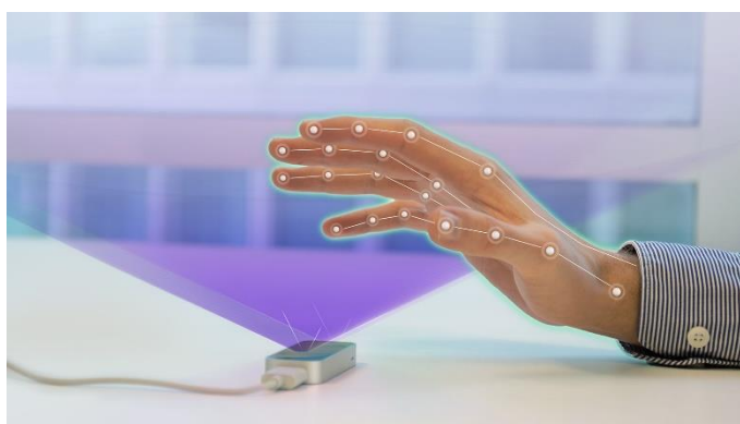
Figure 3. Hand landmarks tracked by Ultraleap devices include fingertips, finger joints, as well as the wrist.
