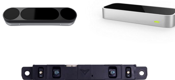
Figure 2. Ultraleap hand-tracking devices. Leap Motion Controller 2 (top left), Leap Motion Controller 1 (top right), Stereo IR 170 (bottom).
